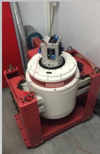
Vibration Ling Shaker with DPA4 amplifier and DSB8 Controller
