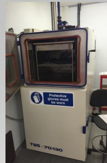
Thermal Shock CTS TSS- 70/130 with TAE EVO 051 Chiller
